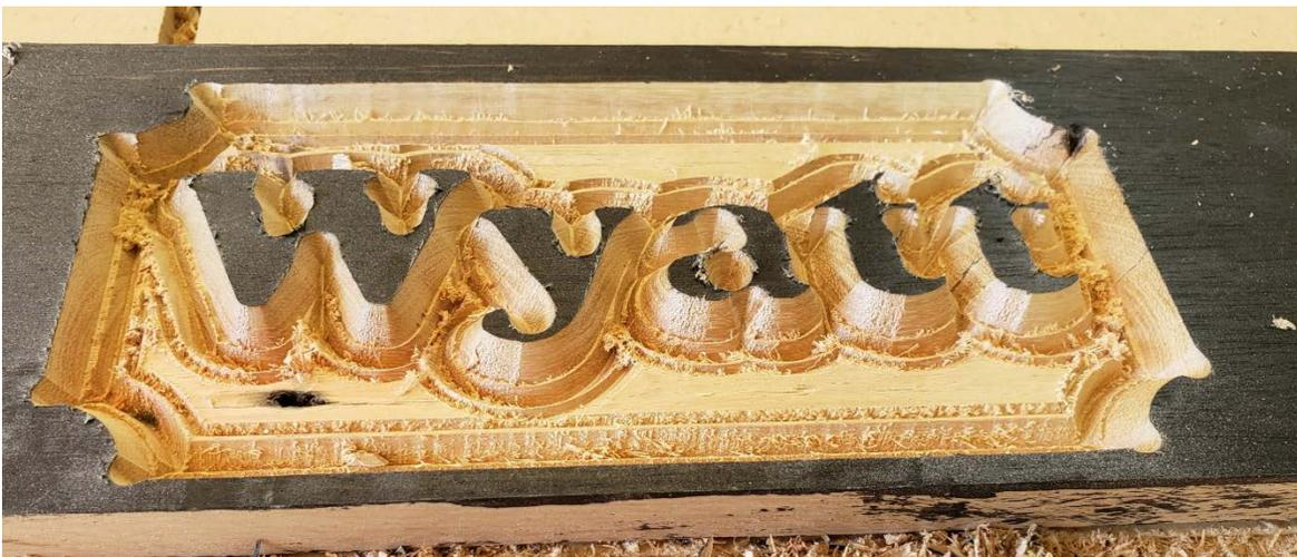
This is the exterior V Bit cut, set to 0.200" and cutting to close to 0.400", which matches the inside V carve depth. It should leave a face surface, as shown in the Vectric image.
