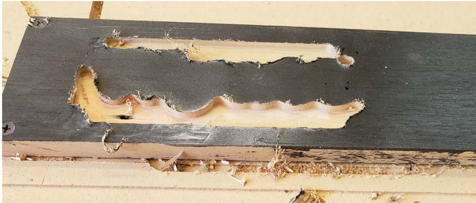
This is the V Carve pass with the Shapeoko Tool 301, 1/2" 90 degree V-bit. The cut is set to 0.200" and the actual cut is close to 0.400". The surprises include the depth, the steps at the bases of the letters, and the exterior dog bone issues on the corners.
