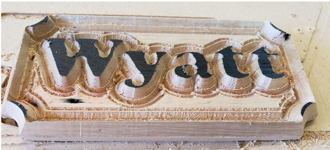
This is the V-Carve Engraving Toolpath set up. The material is 3 1/2" high by 9" wide by 0.525" thick. The desired cut is 0.200.
